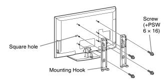
Sufficient expertise is required for installing this product, especially to determine the strength of the wall for withstanding the TV's weight. Be sure to entrust the attachment of this product to the wall to Sony dealers or licensed contractors and pay adequate attention to safety during the installation. Sony is not liable for any damage or injury caused by mishandling or improper installation.
